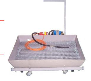
The dirt water recycling collector 1000 KW-FP is used in workshops for cars and trucks to collect, treat, and recycle dirt water which then can be reused in the ph-cleantec machines. The collector is mobile and can be pushed on the ground under (almost) every vehicle. Given its extendable frame with wheels the collector also fits into every pit.
