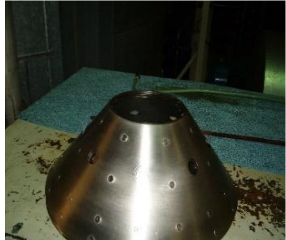
Separators must be cleaned regularly but without damaging the fragile surfaces
